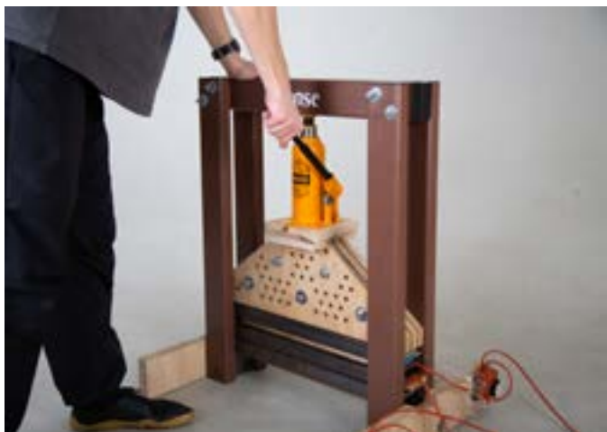
↑ Densification platform, used to compress wood and stabilize through heat. Source: Vicente Carmona.
