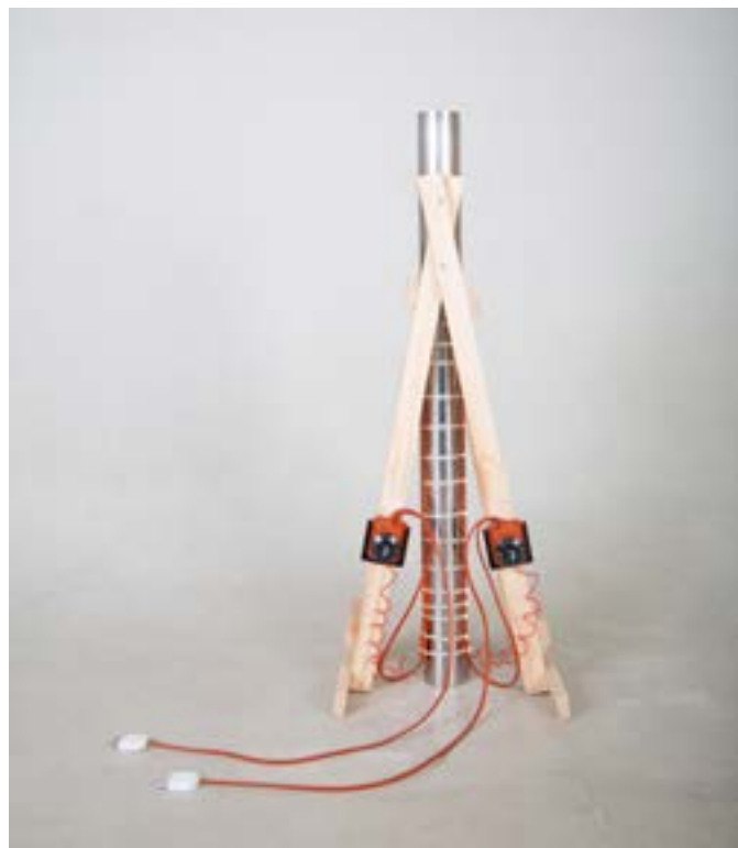
→ Plastification platform, used to soften wood and avoid fracture under pressure. Source: Vicente Carmona.
